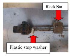
15. Snap the plastic stop washer back onto the shaft next to the gear case. Screw the block nut back onto the shaft.
