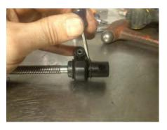
10. Carefully pry the locking rings off each side the gear casing. These rings must be reused.
