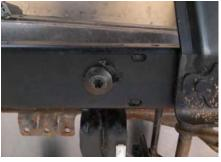
18. Reinstall the floor slides back onto the seat track. Use your markings from step 5 to get each slide onto the correct side and pointing the correct direction. Reinstall the torx head bolts.
