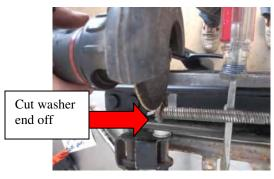
7. Cut the washer end of the shaft off and unscrew the block nut from each shaft.
