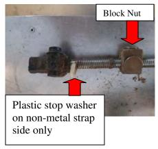
9. Carefully snap off the plastic washer stop. It must be reused.
