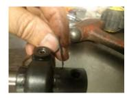
12. Slide the locking rings onto each side the gear casing. Note the inner raised edge points away from the center housing.
