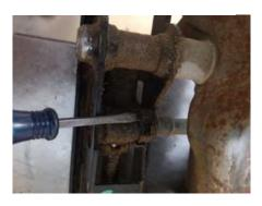
3. Remove both rubber tube holder clips. Be careful not to break off the clip fingers. Leave the rubber tubes attached to each clip
