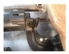
1. Disconnect the black plug from the motor. Remove both ¼ head screws from For/Back motor.
