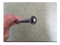
16. Install the plastic washer, metal washer and external snap ring onto the shaft.
