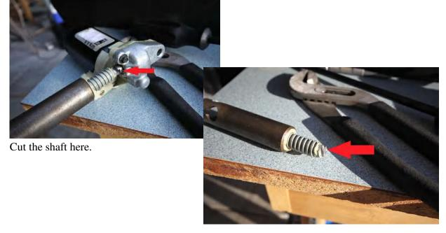
Cut a notch to help unscrew the shaft from the tube nut
