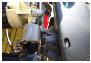
Shows the roll pin after 3/16" is cut off the end.
