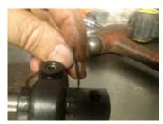
10. Slide the locking rings onto each side the gear casing. Note the inner raised edge points away from the center housing.
