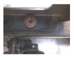
15. Reinstall the floor slides back onto the seat track. Use your markings from step 5 to get each slide onto the correct side and pointing the correct direction. Reinstall the torx head bolts. Do not over tighten the one in the plastic block, it could strip out.
