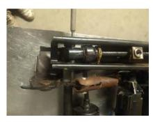
7. Use a small drive pin and drive the roll pin towards the center. You don't have to take it all the way out. If it is easier to drive the pin opposite direction than shown, that is ok. Once removed, lift the gear/shaft out of the frame.
