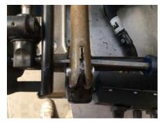
12. Drive the roll pin back into the gear casing. Using various drive pins and screwdrivers might be needed.
