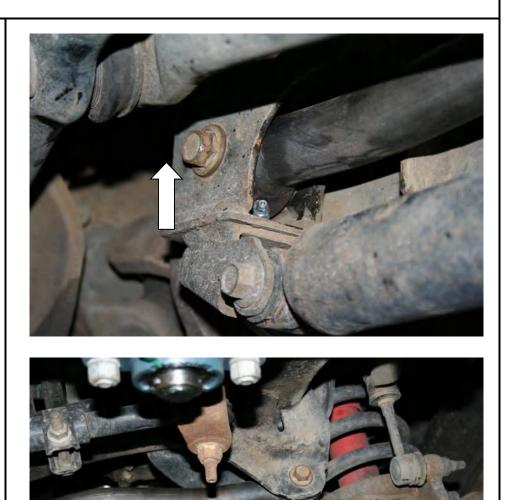
You can now perform an alignment on the front end of the vehicle. Adjust the front axle left and right by turning the threaded connector.
