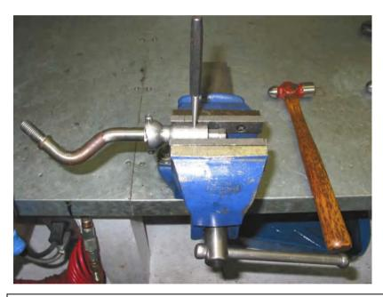
To change the shifter rail pin from the OEM shifter to the BD Short Shifter you will need to remove the shifter rail pin from the shift arm.
