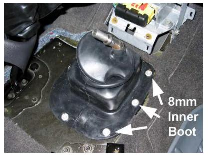
Remove the inner shifter boot with an 8mm socket.
