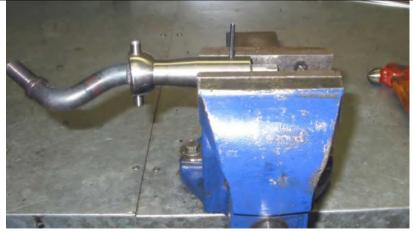
Insert the shifter rail pin into the BD Short Shifter arm and then insert the roll pin with a small hammer. Be careful not to round the end of the roll pin or the shifter rail pin will not be properly secure.
