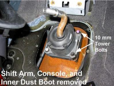
Remove the shift tower from the transmission.
