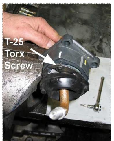
Using a number T-25 Torx bit, disassemble the shift tower.
