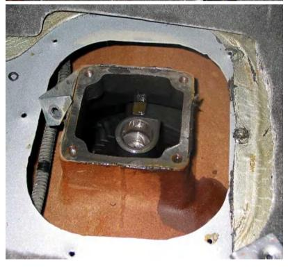
Clean up any residual silicone gasket material from the top of isolator and the transmission case.
