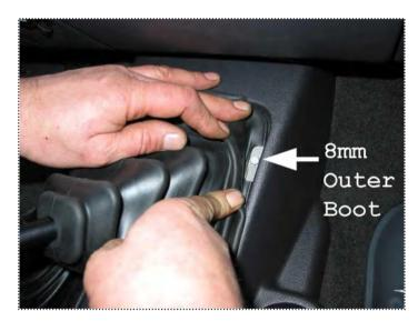
Remove the outer shifter boot with an 8mm socket.
