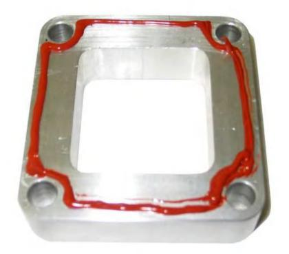
Apply fresh silicone to both sides of aluminum spacer and place on transmission.
