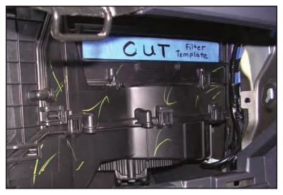
The masking tape template is in place. Time to cut the edges with the "hot butter knife" or Dremel tool.
