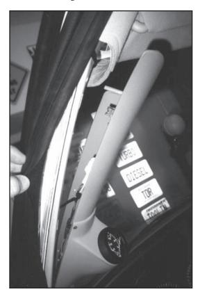
• To route your wires/boost line to the gauges/gauge pod or pillar cover, you will have to remove the plastic A-pillar cover.
