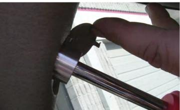
2) Remove the two bolts with a 10mm socket.
