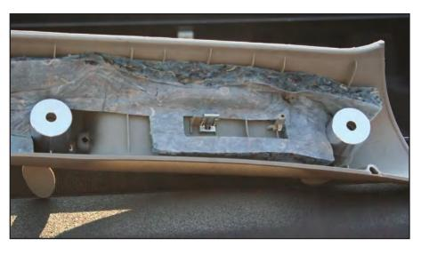
7) Slide the two larger bushings over the stock plastic mount (this is what breaks)
