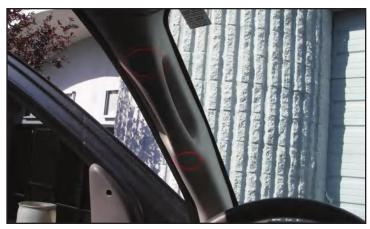
1) Remove Plastic caps with a flat blade screw driver revealing the hidden bolts.
