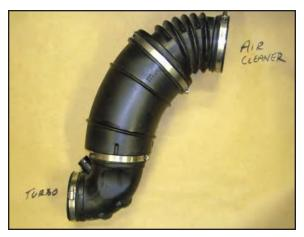
In order to get a better view and better access to plug the block heater cord in, you might find it easier to remove the air intake snorkel.
