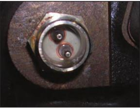
Also, you can see in the picture that the extensions are positioned at 11 o'clock and 5 o'clock. However, the position of the extensions does vary based on how the block heater was installed at the factory.
