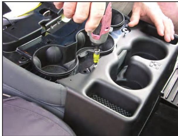
Test fit the cup holder and then screw the self-tapping phillips head screws into place.
