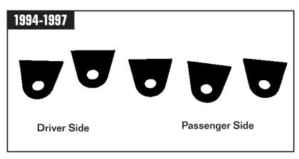
**STEP 3:** Good work! The reinforcement tabs help spread the clamp load and, hopefully, will keep dashboard cracks from happening.
