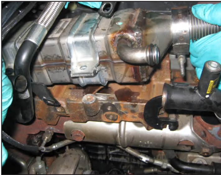
Our task is to remove and clean the EGR cooler assembly. This is the “before” picture.
