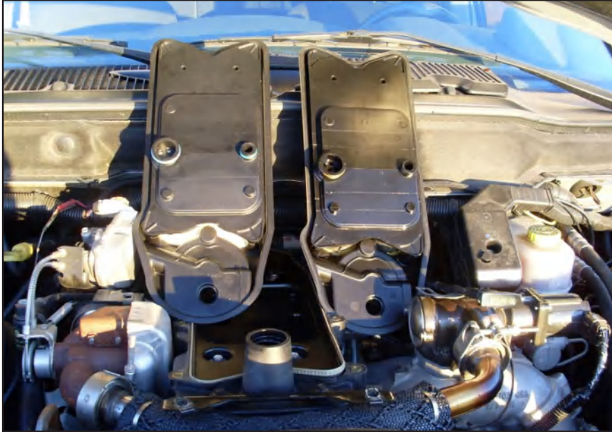
New CCV filter on the left. At 30,000 miles the CCV filter on the right looked clean and was reinstalled.
