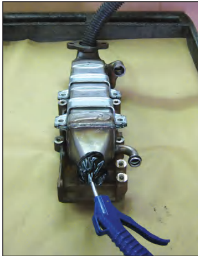
With carefully regulated compressed air you can blow carbon into the inlet hose of a vacuum cleaner.
