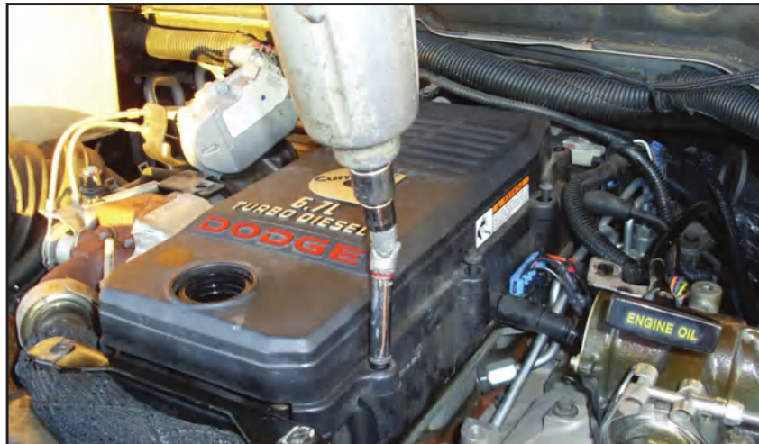
Removing the eight 8mm bolts that hold the CCV filter in place. DO NOT use the impact tool to reassemble and tighten the bolts.
