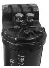
• Bolt the new housing onto cylinder head in same location and torque bolts to 18 foot pounds. You will need to hard wire the new water-in-fuel sensor provided in the kit to the factory harness. Polarity does not matter and this can be done with a variety of different types of electrical connectors of your choice.
