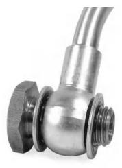
• Install the 4 new 12mm banjo washers in the same orientation as when the original fuel lines were removed.
