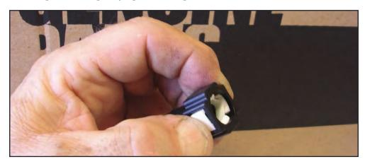
5.) With the Cummins 5253291 fuel line in hand, cut the plastic fuel line and salvage the pinch clips. (We used a slightly heated knife.).
