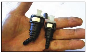
**6.)** With the clips removed from the plastic line, install the clips into the new hose and the 5/16" pressure tee from the kit into the hose. Tighten the hose clamps and reassemble into place. Take extreme care to keep all of the surfaces free of grit as this hose assembly goes after your fuel filter.
