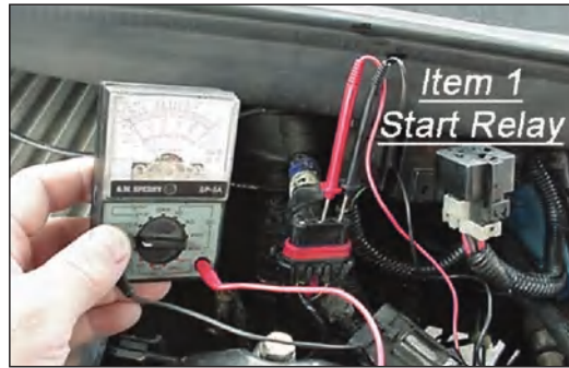
No voltage for “START” tells you to check the relay to the solenoid (Item 1).
