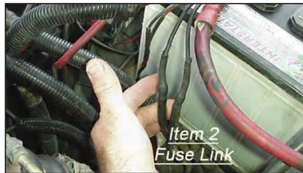
Also check the fuseable link that feeds the solenoid (Item 2) or fuse #9 in the fuse panel.
