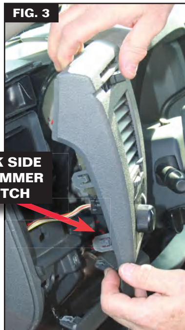
Pull dimmer switch panel back for access to the wiring harness.
