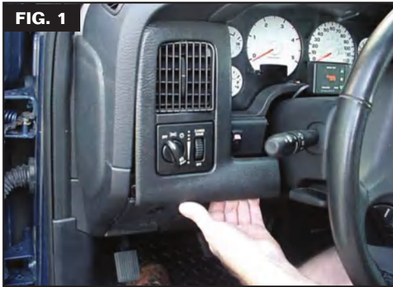
The light dimmer switch is easy to access as the cover and switch assembly are held in place with expansion clamps. Start at the corner next to the steering column, then pull outward.
