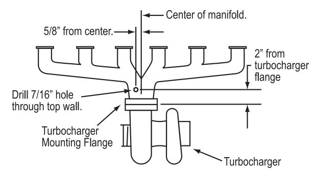
Locate a point two inches from the turbo mounting flange centered on the exhaust manifold, then move forward or rearward on the manifold 5/8," then center punch for drilling. If you are using a 1/4 NPT probe, drill a 7/16" diameter hole straight down through one wall. If you have a 1/8 NPT probe, drill a 5/16" diameter hole. Putting axle grease on the drill and tap will help prevent shavings from falling into the manifold. Tap threads using 1/4 NPT pipe tap or the 1/8 NPT pipe tap.
