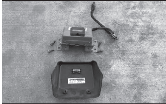
Air bag module and cover. The snap attachment of the cover and the four mounting bolts are shown.
