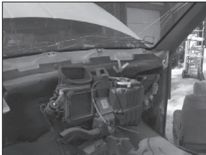
Another view of the HVAC box with the dashboard assembly removed. Two mounting nut positions are indicated by arrows.
