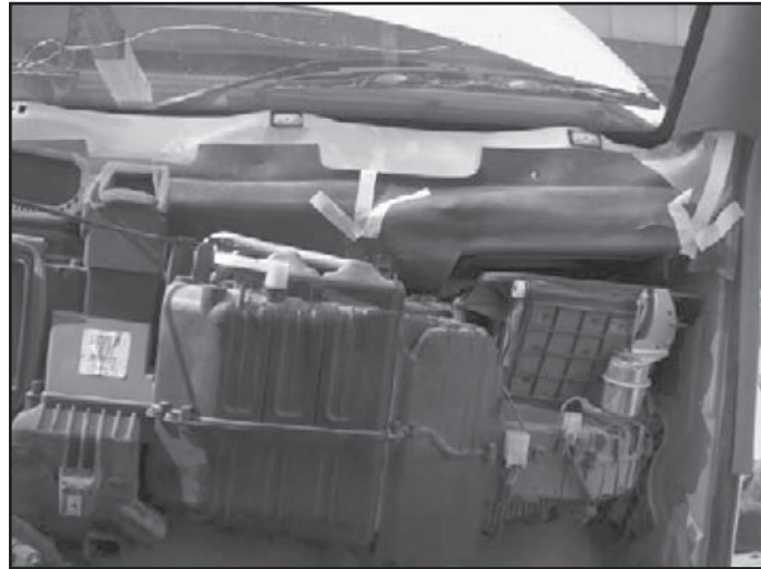
View of the HVAC box with the dashboard assembly removed. Two mounting nut positions are indicated by arrows.
