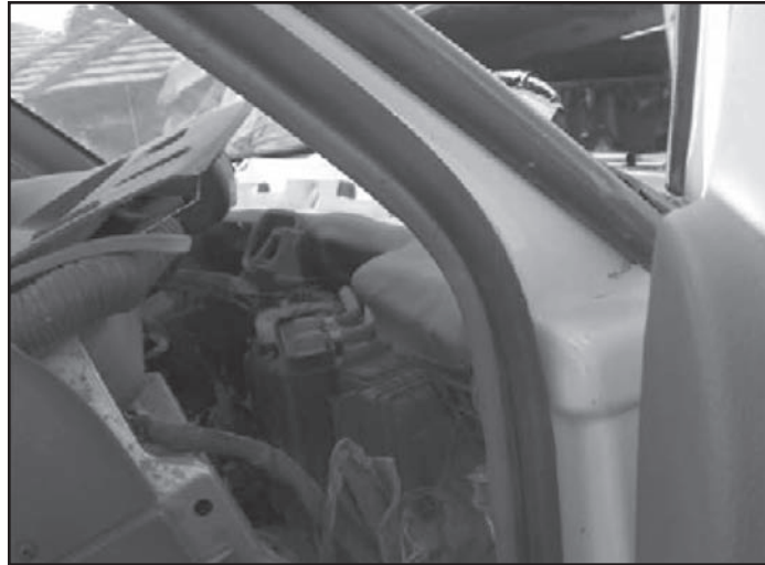
Extent of access to the HVAC box is shown here.
