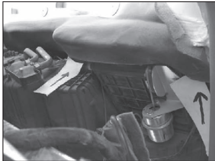
View behind the dash of the HVAC box. Two mounting nut positions are indicated by arrows.
