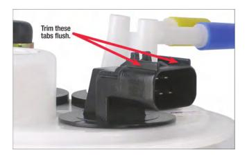
2. Test fit/plug in your adapter. Again, polarity of the two black connector wires does not matter. If you choose, verify continuity with a volt meter. Finish the installation. Thank you for your purchase.
