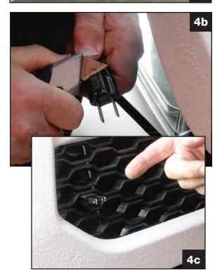
Choose a place where it will be easy to access the male three-prong connector. In picture 4a we located the male connector by the tow hook. In picture 4b we took a knife and whittled away some of the plastic and eliminated the ground prong so that it would fit into a grille slot shown in picture 4c. Placement of the connector is yours to choose.
