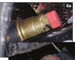
Remove the red dust cap from the block heater shown in picture 5a. Note the orientation of the cap as shown in picture 5b. You will want to hold the heater cord in the same direction as shown in picture 5c.
