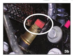
Picture 3b is a close-up photo showing you that the block heater comes from the factory with a little red cap. Do not remove the red dust cap just yet!
