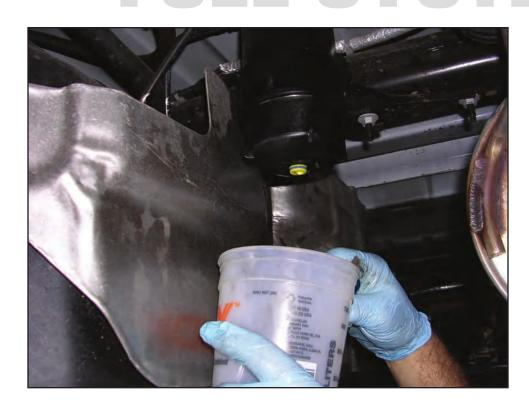
Now, with the canister, fuel filter and diesel fuel baggie or bucket removed, let's take a look at the yellow (lack of drain) drain plug. Because it has a "T" shaped head, the plug doesn't drop out of the canister. When it is unscrewed it just doesn't have the right cuts in the plastic to allow fuel to drain.
