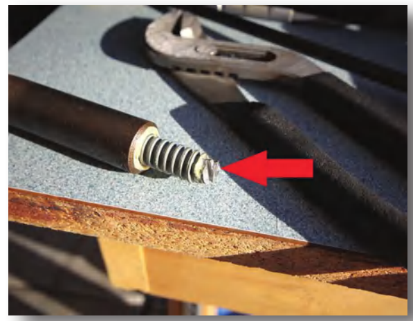
Cut a notch to help unscrew the shaft from the tube nut.
