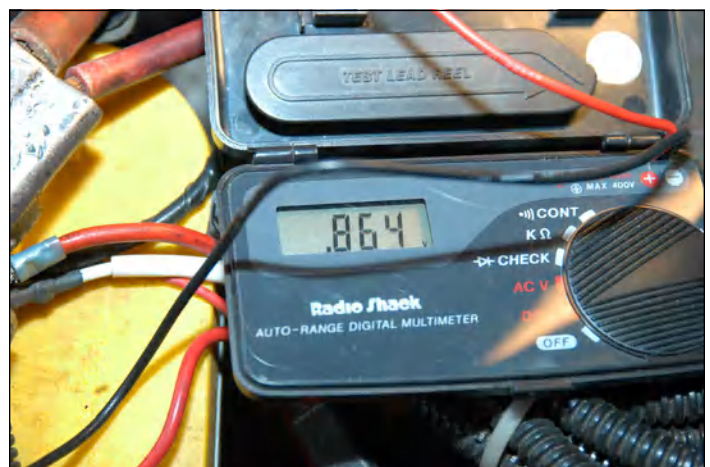
My line voltage at idle (key on, engine not running) was .864 volts.
