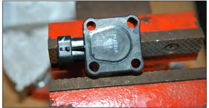
Using a 3/16" rat-tail file, I slotted the two mounting holes allowing for more rotation of the switch.
