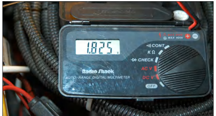
I now have 1.8 volts at the "idle" position of the TPS.
