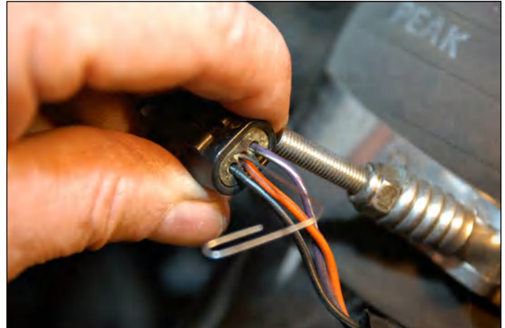
A sharpened paper clip inserted into the center position of the connector.
