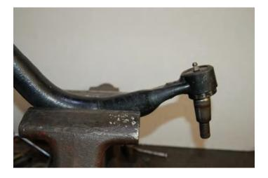
**Step 3**: Removing Ball stud from track bar. Please identify which track bar you have. See front page to identify. If it is the Dodge bar, please go to Step 4, if you have a NAPA bar continue on to step 3A. This is very important. Failure to do this could cause problems in installation.
