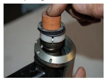
**Step 9**:Now install the threaded nut and tighten by hand until it wont go further. Then tighten with ½ inch drive ratchet until tight. You will feel it bottom out. This is generally about 35lbs of torque.
