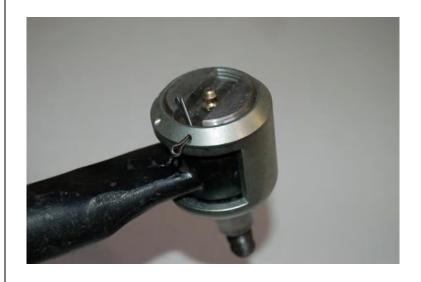
Adjusting A Luke's Link Track bar kit. Luke's Link comes with 3 small metal washers. These are used for adjusting the Luke's Link in case steering gets a little loose (wonder). To adjust, leave truck on ground with steering wheel unlocked, remove cotter pin and unscrew plug. Put one spacer under spring. Replace plug and cotter pin. This will take up the play in the end.
