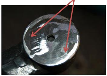
**Step 5:**Break loose encasing seal. With bar in vice as show, hit with hammer to break loose. Usually 2 or 3 hits will break loose. Remove parts from inside bar and throw away. There is metal Race under ball stud, if it falls out, please put back in. Do not damage ball stud. It must be reused.
