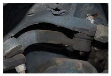
**Step 2**:Remove track bar from truck and secure in vice as shown. At this time remove grease zerk.
