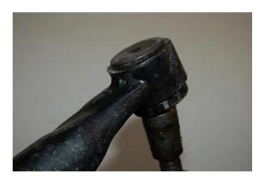
Step 6: If cap does not slide over bar, you must continue to grind until cap slides over, do not force cap over end. Please note
