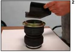
**3** Using the two <sup>3</sup>/<sub>8</sub>" NF x <sup>7</sup>/<sub>8</sub>" capscrews, flat and lock washers, loosely fasten the assembly together. Do not tighten the capscrews fully until final adjustment is performed in step 8.
