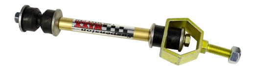
4. Install supplied lock washer and start retaining nut Continue on opposing side. Install upper sway bar bushing, washer and nut. Tighten to lightly compress bushings (tighten so approximately 1/4" - 3/8" threads exposed) See Recommended Compression Guide. View MAXXLink and rotate as needed to center lower concave /convex bushings. Hold MAXXLink in place and torque retaining nut to 60 ft/lbs.
