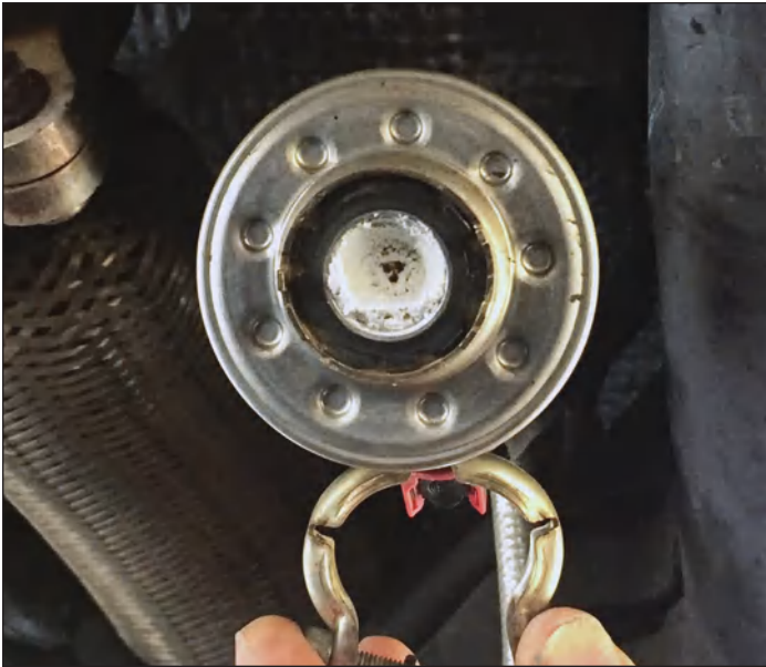
It is held on with an expanding collar. A 4mm hex head was used to loosen the bolt. Next you expand/remove the collar. You can see the collection of white crystal material on the injector.
