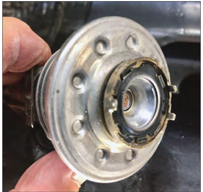
With the approved service tools (hot water and an old toothbrush) the white crystals were removed. I also cleaned the spray passage into the exhaust. Nice injector! Notice the three alignment tangs on the injector. Align, reattach the expanding collar and bolt it back on. Service time, 10 minutes (cold).
