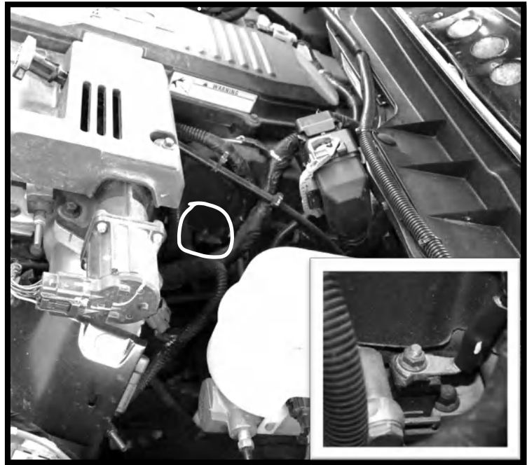
Above: Location of stud shown (circled) under the hood. Detail of nut in the inset.
