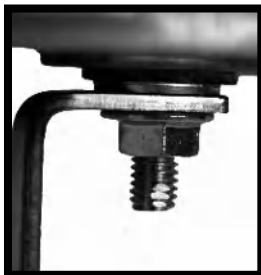
In the photo to the left, you can see that Ram has machined a flat spot onto the threads to help prevent it falling off. (This view is from the underside of the intake plenum).
