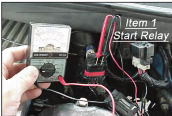
No voltage for "START" tells you to check the relay to the solenoid (Item 1).
