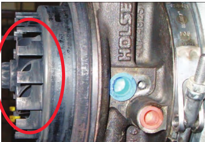
With the sleeve fully extended, the vanes are closed to exhaust flow. This creates exhaust gas back pressure (the exhaust cannot escape) and the turbo acts like an exhaust brake.
