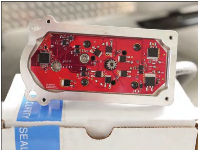
City Diesel's VGT circuit board is designed to withstand higher temperatures than OEM.
