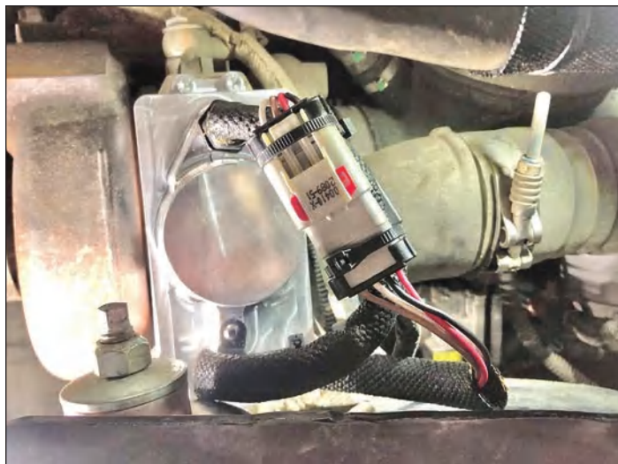
Wiring harness is longer than needed for my application, but secured, zip-tied, and tidy.
