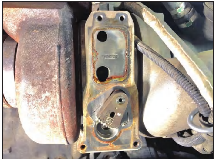
Stock Holset actuator removed for the first time. Turbo actuator gear lever at bottom must not be seized.
