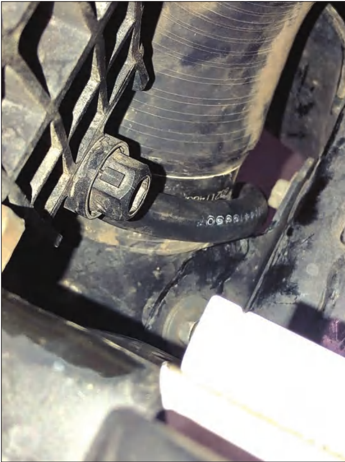
Radiator drain tube fitted. A new stubby 16 mm was helpful to open and close the drain.
