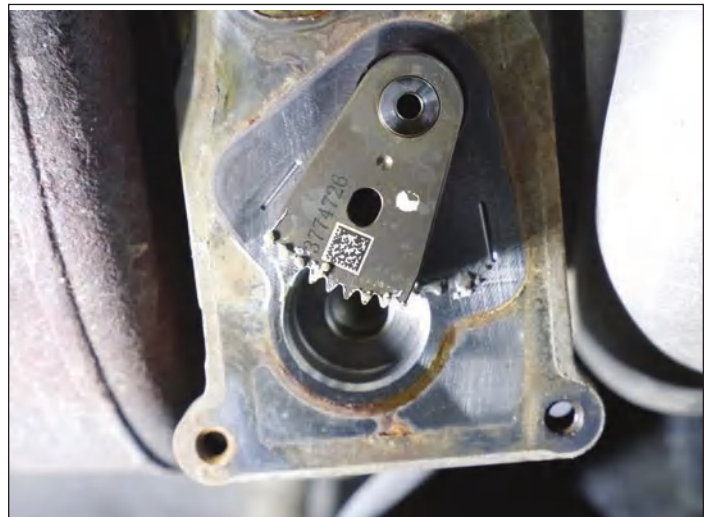
Closeup of turbo actuator gear lever. Ensure it still works before breaking the security seal on the new actuator parts.
