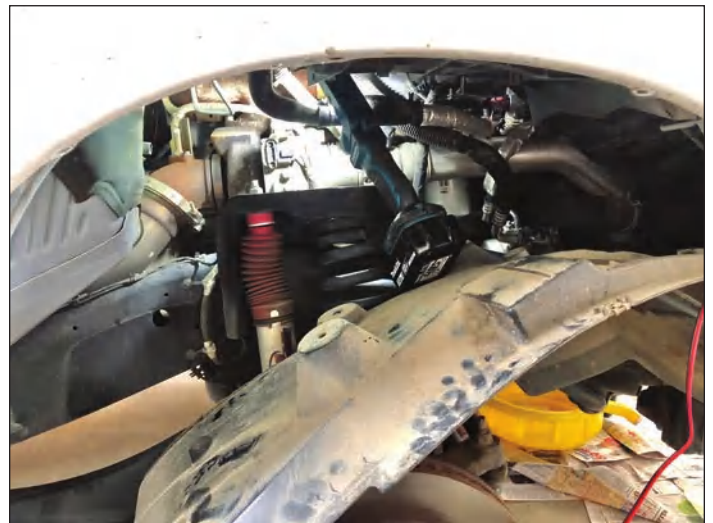
Fender liner dropped (front still attached) to reach the actuator.
