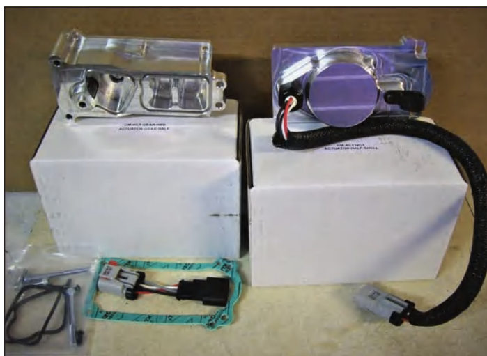
This photo shows the opposite sides of the City Diesel actuator. Both halves are machined from billet aluminum, not made of castings like the Cummins OEM parts.
