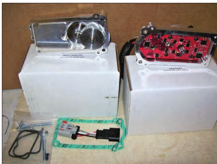
The City Diesel gearbox on the left, and the electronics and drive gear module on the right. This photo shows the halves that mate together, with the gasket and controller cable adapter below.
