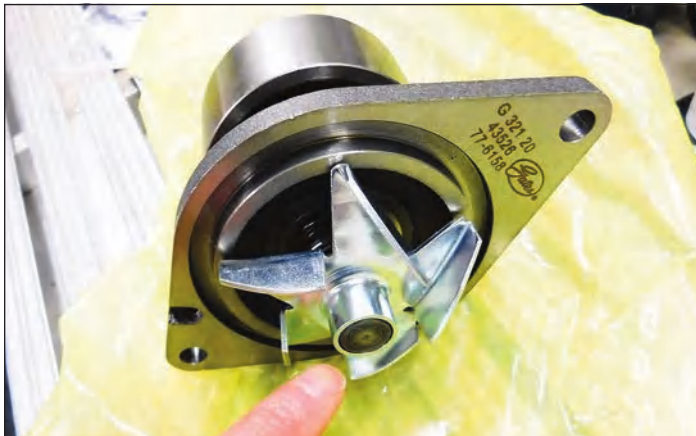
The 43526 Gates pump still looks ruggedly built and cast nicely with good machining. The impeller shaft, however, fits flush with the end of the impeller hub. On the earlier pumps and in ad photos for the 43526, the shaft protrudes through the impeller.
