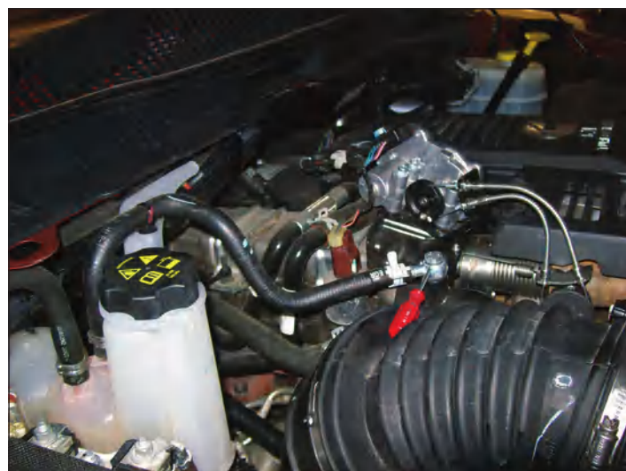
2013 coolant reservoir on left, red-handled screwdriver pointed to high-fill point banjo bolt.
