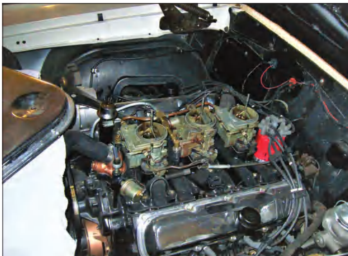
Factory triple two-barrel carburetion on 1966 Oldsmobile 4-4-2.
