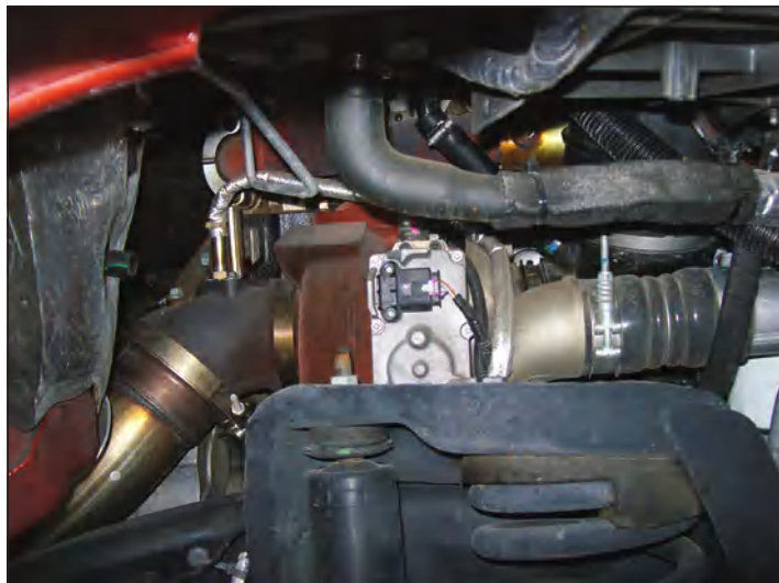
View of turbocharger and actuator with inner fender removed. Access to lower actuator mounting bolts is restricted by the shock absorber/coil spring tower.
