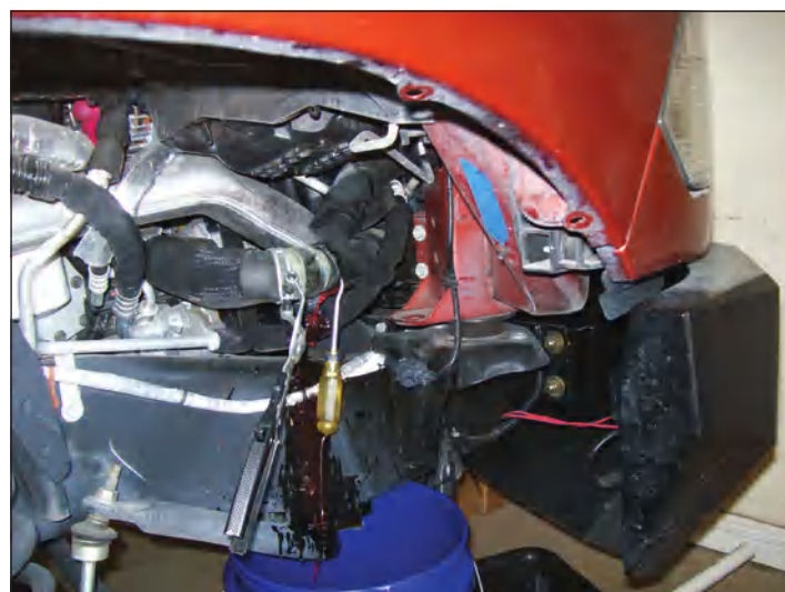
Coolant draining with ratcheting retainer clamp pliers and cotter pin removal tool between hose and plastic Y. Front Christmas tree retainer position is shown with blue arrow.
