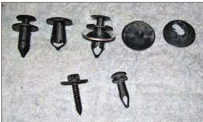
Jeep-style removable plastic fasteners open (head out), closed (head popped into base), and with 1" diameter washer. To the right are the inside of a Christmas tree fastener head and one that has been ground off with a die grinder. At the bottom are the sheet metal screw and the retainer for the bottom of the plastic trim at the rear of the wheel well.
