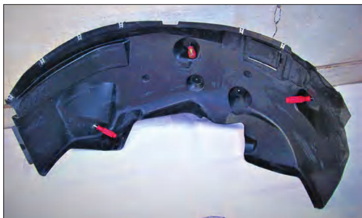
Tire side of inner fender with red-handled screwdrivers in the three "Christmas tree" positions.
