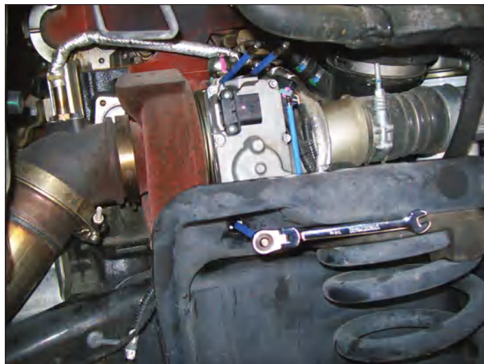
Blue tape-wrapped power bits on top two and bottom left actuator bolts. 5 mm allen key on bottom left actuator bolt. Bottom left bolt is easily accessed through hole drilled in shock absorber/coil spring tower.
