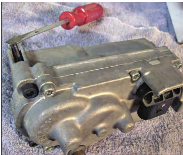
Stock Holset turbo actuator, with red-handled screwdriver pointing to the exposed left lower bolt from the cut-away design of the actuator housing. Here is where dirt, salt, and water enter and corrode the bolt into place.
