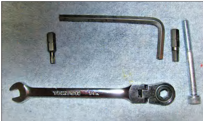
5 mm Allen wrench at top, 1/4" ratcheting box end wrench at bottom, City Diesel actuator bolt at right. Two short bits, tamper proof on left and 5 mm on right from Geno's.
