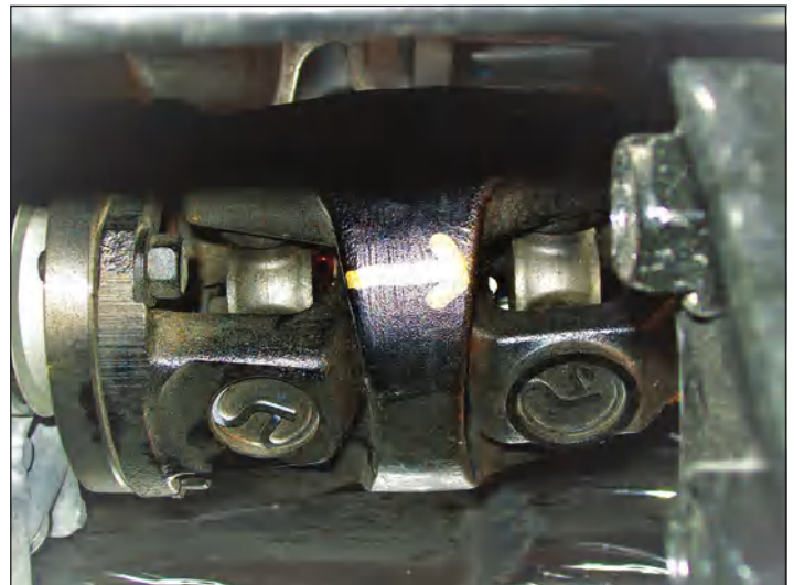
Front driveshaft double cardan joint with arrow pointing to the flush-mount grease fitting.
