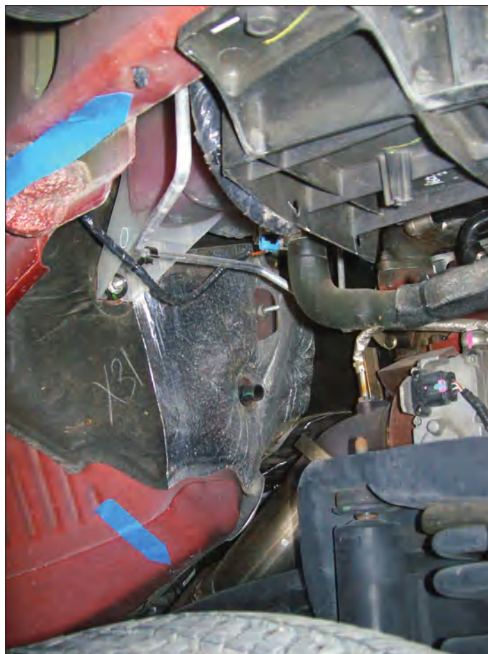
Blue arrows show rear and middle Christmas tree fastener positions. Turbo and actuator can now be seen.
