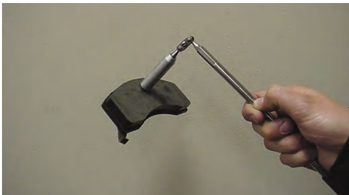
Shown are Hawk-brand semi-metallic brake pads. They passed the magnet test.
