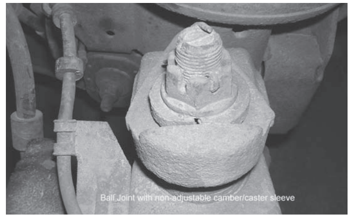
Ball joint with non-adjustable camber/caster sleeve.
