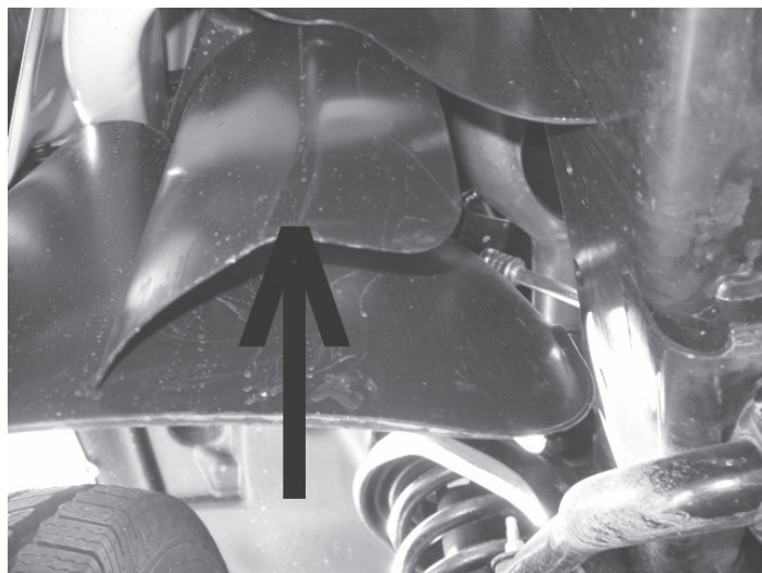
Arrow pointing to vertical baffle used on '04.5 and newer trucks to keep under-hood heated air from entering the air box
