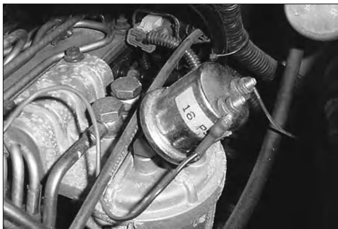
The Westach fuel pressure sending unit mounted on a '98.5/'99 model engine.
