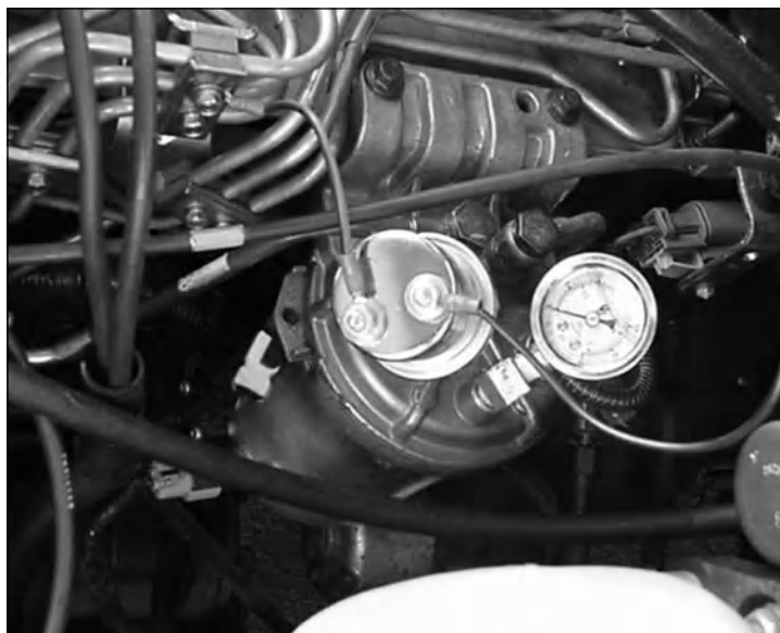
In the photo, note that the Editor's truck (a '99 model) is outfitted with two gauges—one is a mechanical, liquid-filled gauge and the other is a Westach electrical gauge with a pressure sending-unit mounted to the filter head assembly.
