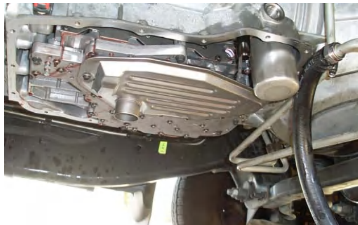
The bottom cooler line is the return-to-transmission line. Remove it with a 1" open end wrench. Clamp a 3/4" ID hose over the threaded barb and direct the fluid into a 5-gallon bucket.
