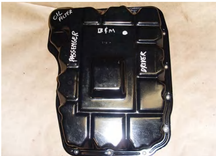
From my study of the internal parts of the 68RFE, I determined that the best place for the drain plug was the location that I marked "B&M."
