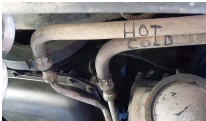
A view of the transmission lines from the front of a Second Generation truck. Follow the "cold" line back to the transmission cooler and disconnect the line at the junction point. Attach your purge hose to the metal flare at the transmission cooler.
