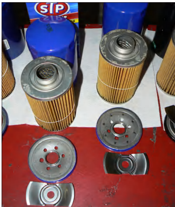
Inspection of the STP filter shows the limited number of holes in the base plate, the stamped metal spring to preload the cartridge, and the minimal number of pleats in the filtration media.
