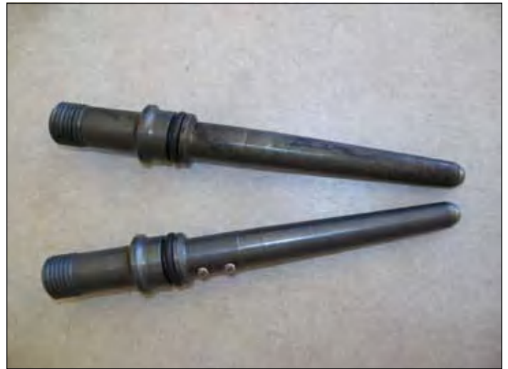
72i13 Rust pitted connector tube above a good tube.
