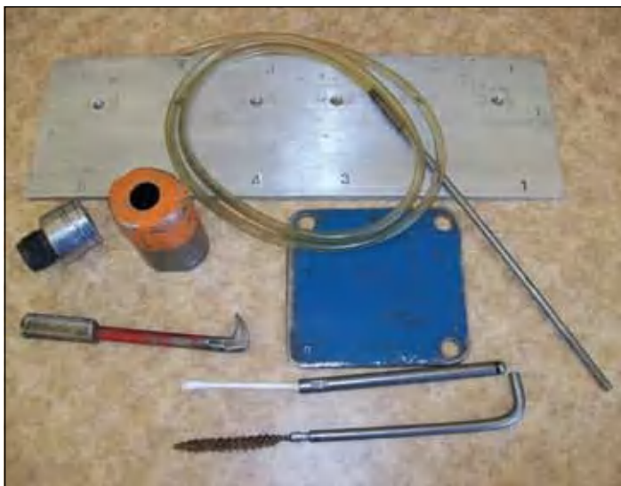
72i20. Specialty tools for HPCR injector replacement.
