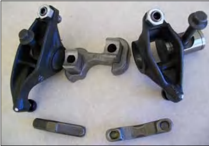
72i21. Rocker assembly for one cylinder. Exhaust, pedestal, intake, rocker pivot shaft and bolt, and two bridges below to couple pairs of intake or exhaust valves.
