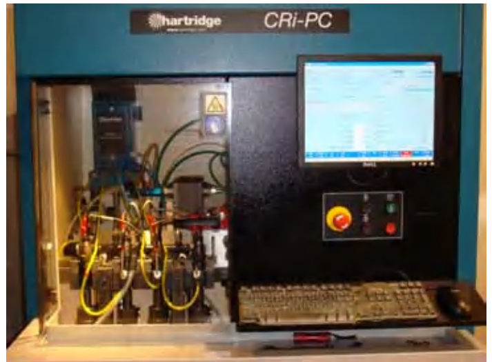
72i9. Hartridge injector tester to determine leakage, flow rate, and response time
