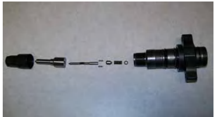
72i16. Disassembled bottom half of HPCR injector.
