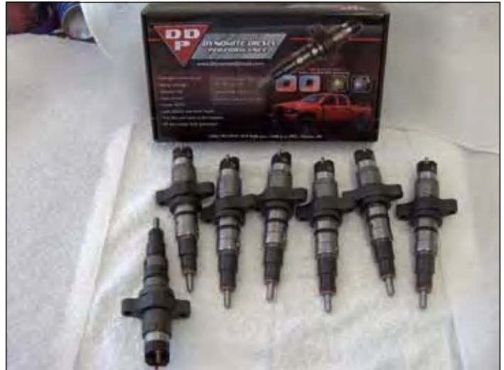
72i11. Six new DDP Stage 1 injectors with the new Bosch shiny white coated steel bodies. Facing the other way is a used injector with the regular gray colored steel body.
