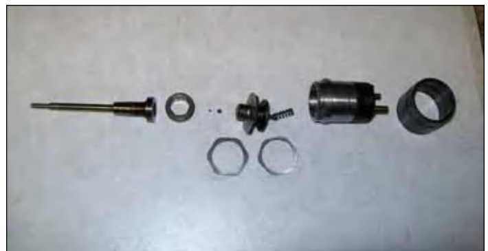
72i17. Disassembled top half of HPCR injector.
