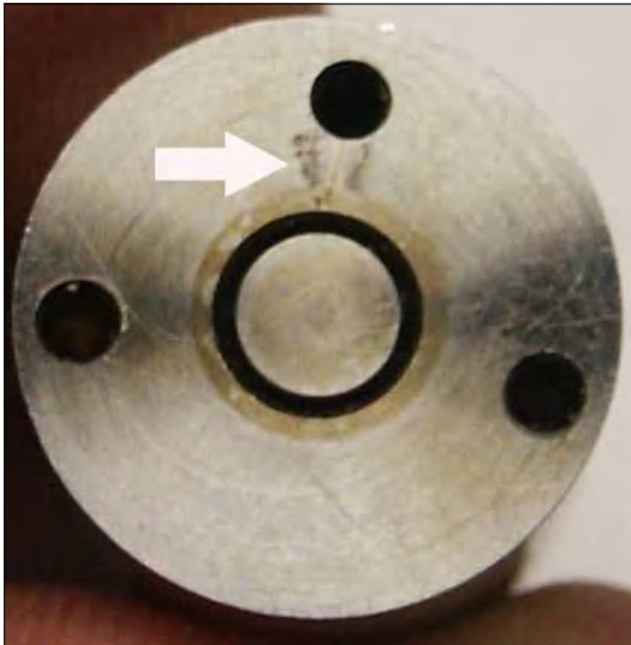
72i14. Cracked injector nozzle
