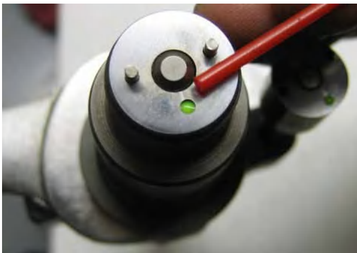
72i15. Cracked injector body
