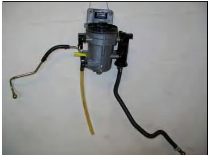
72i5. The electric fuel transfer (lift) pump used from 2003-4 is on the side of the fuel filter canister that faces the rear of the engine. The 2005-up models use a fuel transfer pump mounted inside the fuel tank.
