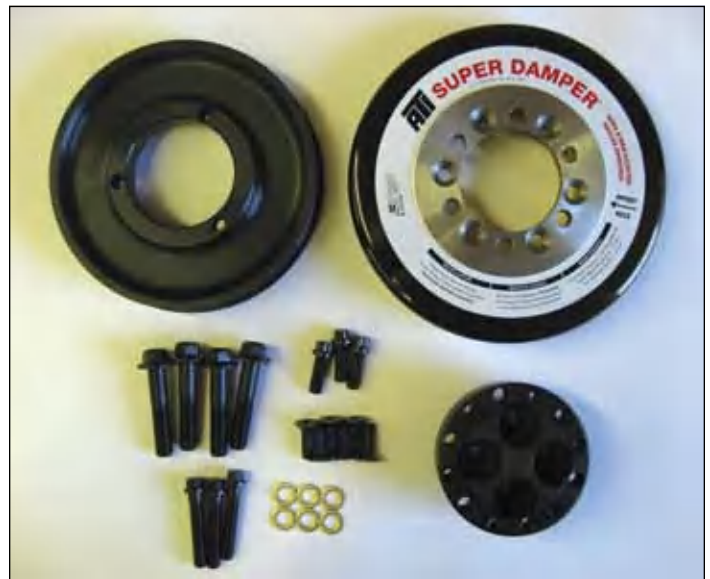
The ATI Super Damper is supplied in three parts: the damper itself, the vehicle-specific hub, and the aluminum pulley. All necessary bolts and screws are supplied to assemble this damper, but it cannot be assembled before installation on the engine, due to the fact that the installation bolts do not fit through the crankshaft flange holes after it is assembled.
