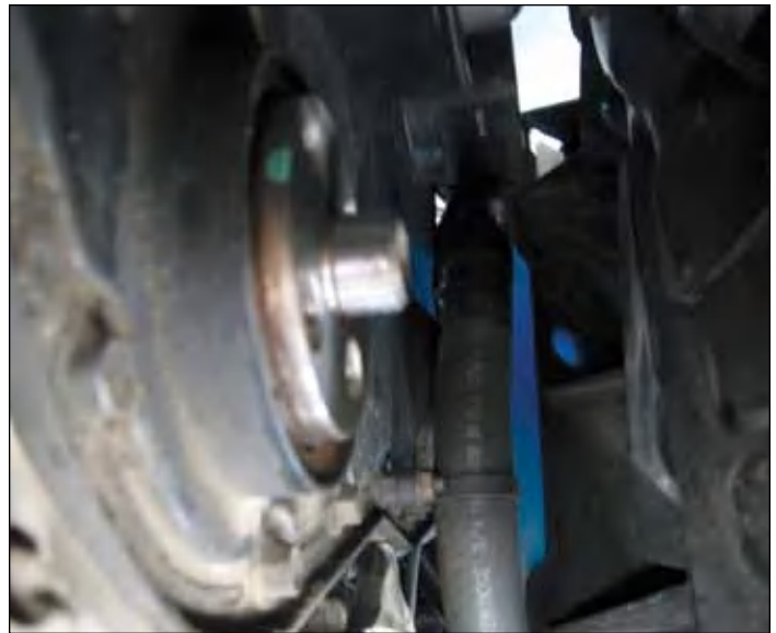
The damper is hub-centric and is aligned on the extension that is machined on the end of the crank. It is important when installing whichever damper you use, to use anti-seize or grease on this hub when fitting the new damper so as not to gall this close-fitting surface when turning the hub for bolt alignment.
