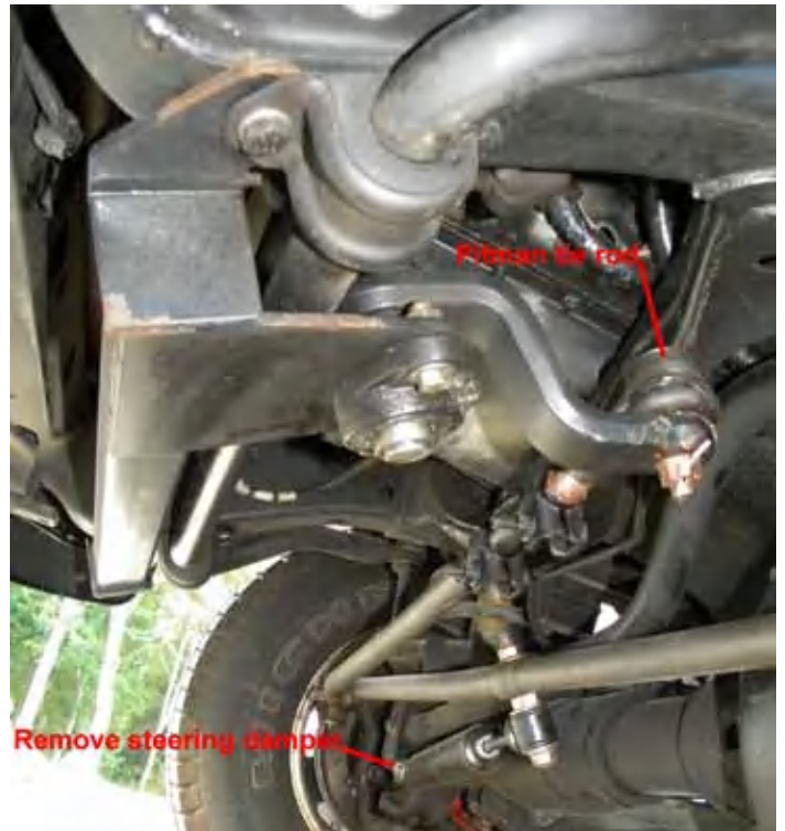
Remove steering damper.
