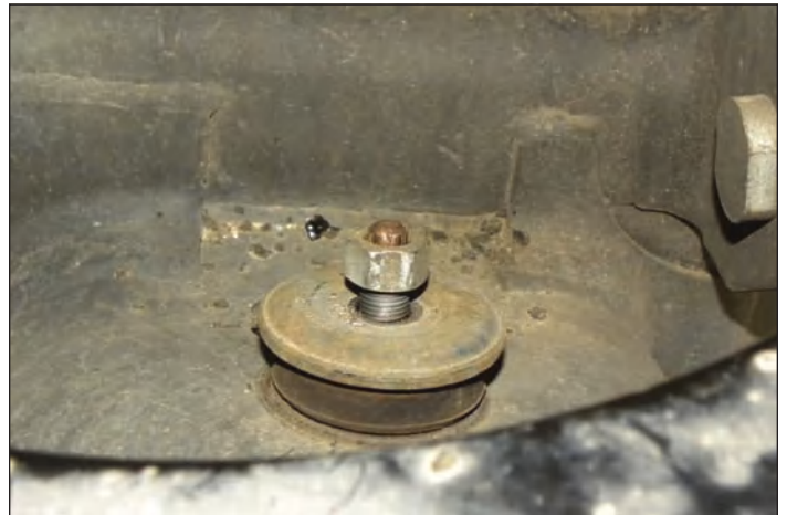
Note top of shock stud has flats for holding with 9mm wrench while large nut is loosened with 18mm wrench.
