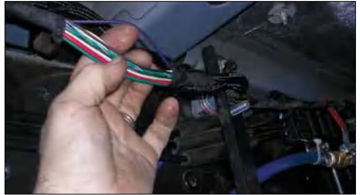
Intercept the wiring harness at the area of the driver's door and you can manually operate the fuel transfer pump.
