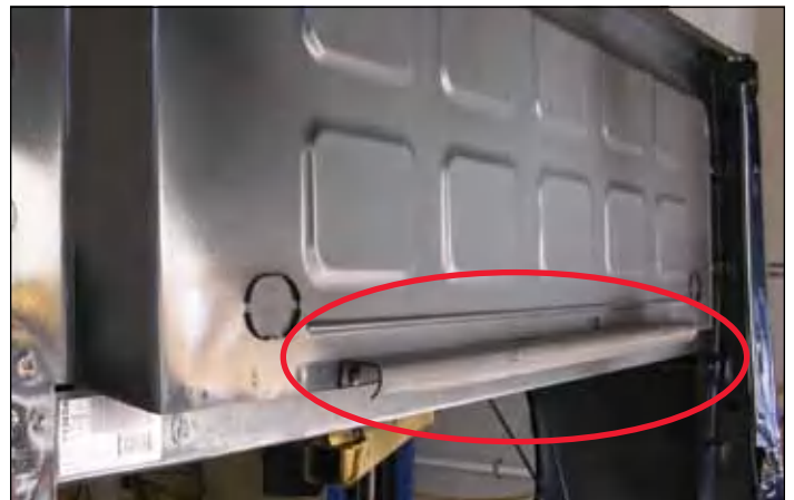
The truck's plastic bed snubber.
