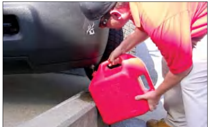
Utilizing the fuel drain line extension tip from Issue 75 it is easy to drain the fuel tank.
