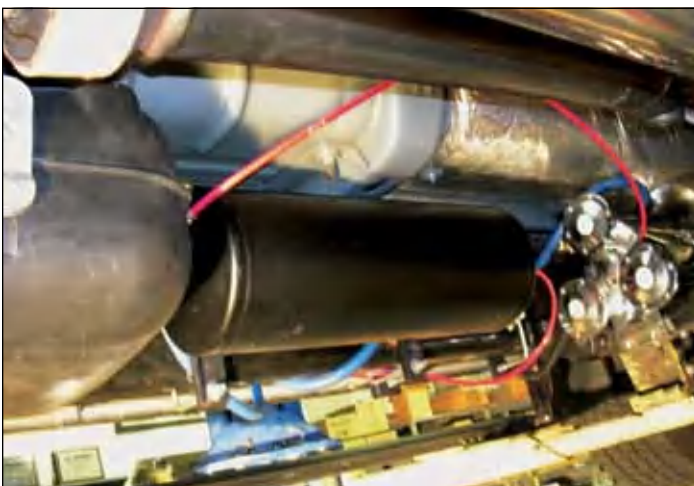
The inside of the driver's side frame rail holds an air tank and air horns.
