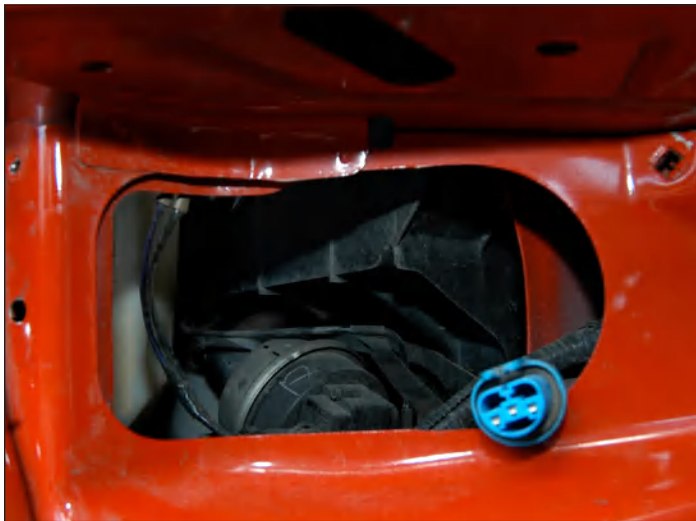
The light pocket in my '98 Turbo Diesel already has the cut out needed to install the Sport lights.
