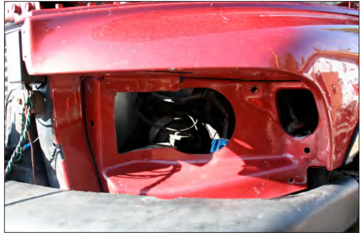
Our Canadian Turbo Diesel was not so fortunate and needed to have the cut out made to accommodate the Sport lamps. A Sawzall works well. Be careful not to cut out the ground lug. Be sure to paint the cut edge to prevent rust.
