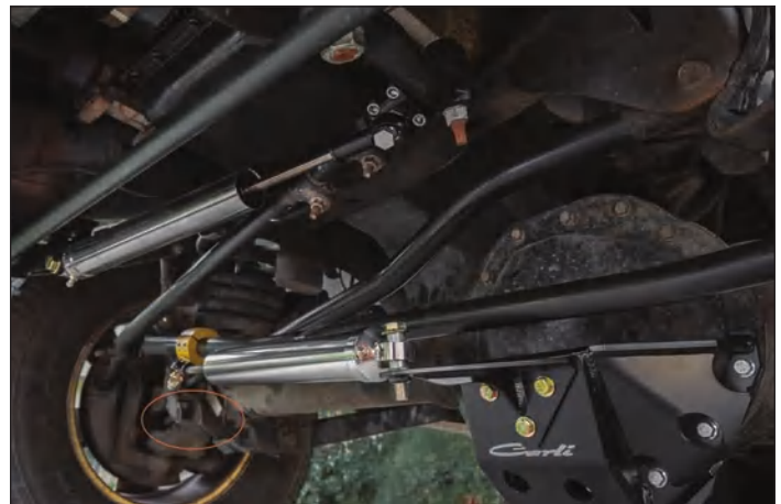
Figure 3: My (Issue 87) Installation of the Carli Suspension "Dual opposing steering stabilizers." Without using the factory mount point, the lower stabilizer is located above the bottom of the axle tube, reducing the risk of damage in off-road situations.
