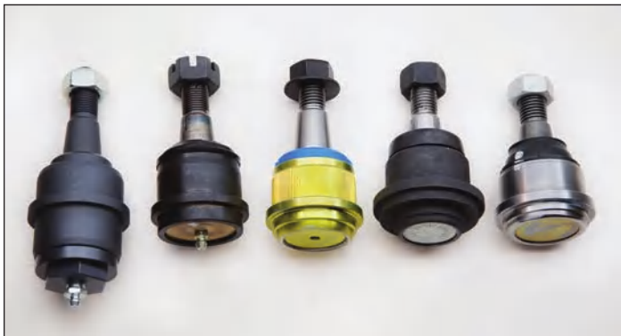
Figure 1: from left to right: Upper ball joints from Carli Suspension, Moog, Napa, Duralast, and Mopar. Some are smooth, some are knurled, some have a grease zerk, and some are sealed. The Zerk on the NAPA part in this photograph has not yet been installed.
