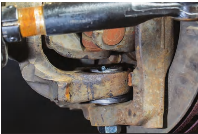
Figure 5: The Carli Suspension Lower Ball Joint, installed at exactly the right position so that the grease zerk is accessible.
