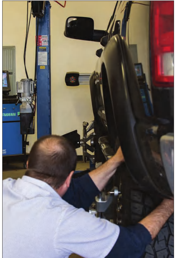
Figure 6: Four wheel alignment in progress at Auto Works automotive repair in Coeur d'Alene, ID. In this photograph, Troy Hocking is rolling my truck back and forth several inches at a time, to check wheel runout. All parameters including camber, caster and caster sweep, checked out.
