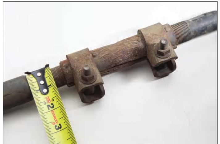
Figure 6: My tape measure shows the 1.25" diameter steering linkage tubes used on the 2003-2008 "Y-type" steering system that I replaced. The newer "T-type" system uses larger 1.5" diameter tubes.
