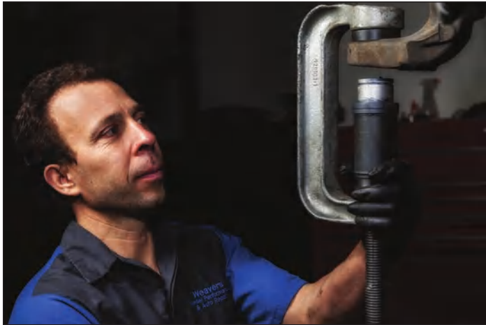
Figure 4: Raymond Driggs at Weaver's Diesel Performance, installing my lower left ball joint.
