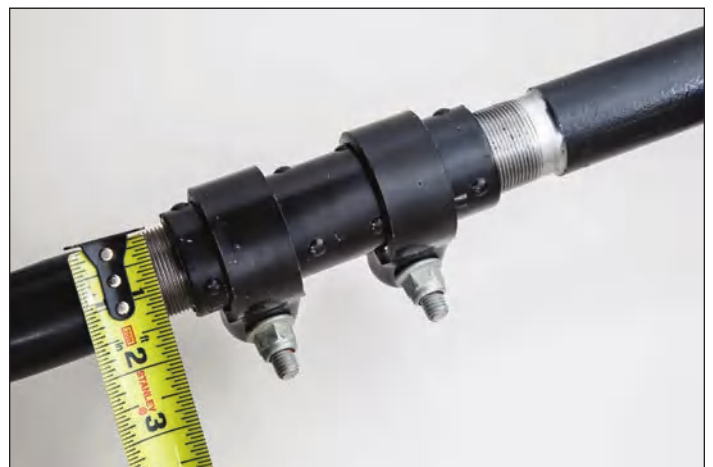
Figure 7: T-type steering system is made with 1.5" diameter tubing, and is considerably more robust than the older, Y-type steering system. The new system is over five pounds heavier.
