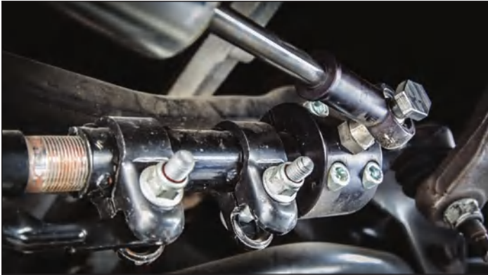
Figure 12: Installation of the Carli Suspension "High mount stabilizer" required a new clamp to accommodate the new tube diameter.
