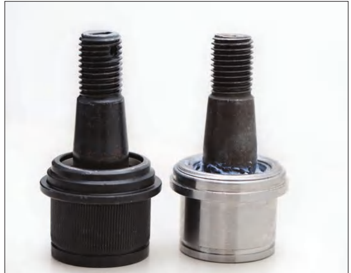
Figure 2: Lower ball joints from Moog (left) and Mopar (right). The Moog "problem solver" part supplied by my local O'Reilly Auto Parts store has a knurled body.
