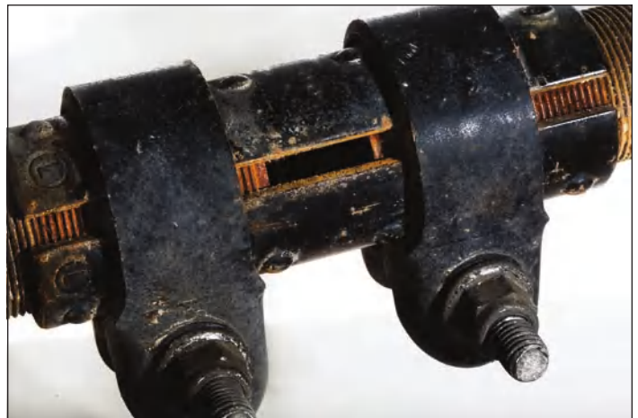
Figure 12: The older (recalled) system allowed the right hand tube to rotate along with the adjustment collar, allowing a careless technician to pre-stress the ball stud inside the steering knuckle.
