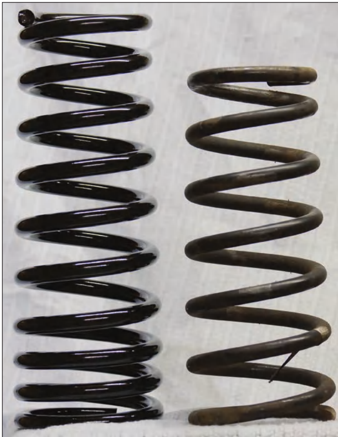
Figure 1: Carli Suspension multi-rate coil spring (left) installed in 2012, provided approximately three inches of lift compared to the factory spring (right)
