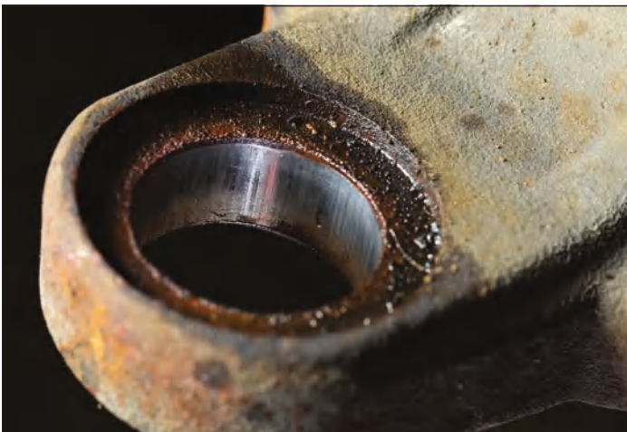
Figure 3: The smooth lower ball joint knuckle bore on my Turbo Diesel. I decided not to install a knurled or oversized part, in order to preserve the factory bore as long as possible.
