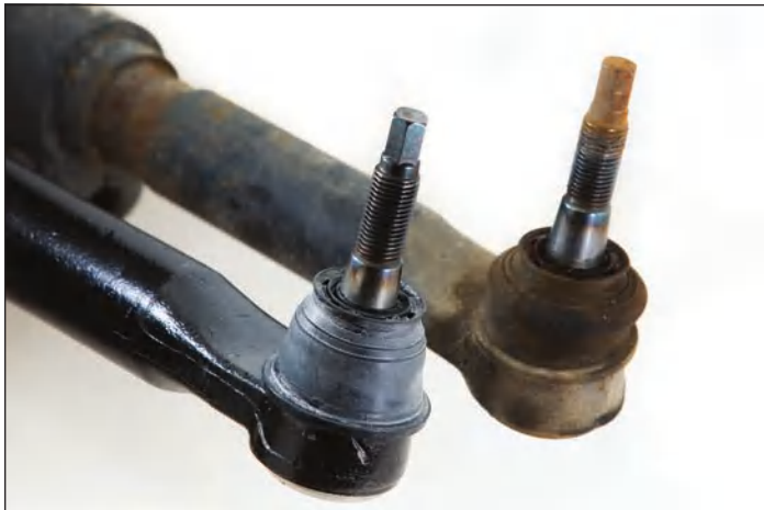
Figure 10: I found no difference between "good" and "recalled" tie rod ball studs, the subject of N49. On the left is a verified "good" part which I installed on my truck. On the right is a recalled part from my dealer's boneyard.
