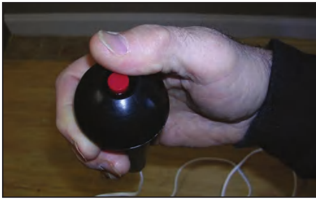
Those with a manual transmission can use this gear shift with a switch at the top to turn on/off the exhaust brake. Trick, eh?
