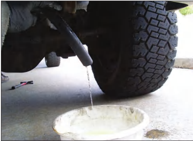
Extend the fuel filter drain hose to save the aggravation of having the fuel drain onto the frame which is caused by the existing short drain hose.
