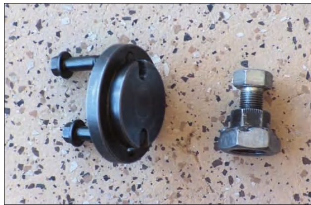
T6. The Snap-on SP504 gear puller with M8x1.25x40 bolts and the home-made pump shaft turning tool at right.
