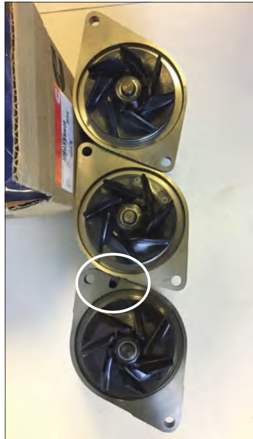
The official T512AA water pump is on the bottom. We circled the weep hole which sets it apart from the other two pumps.
