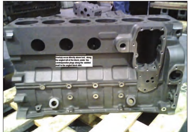
Crack(s) occur directly above text, along the angled rail of the block, under the core/expansion plugs along the molded shelf to the angled block skirt.
