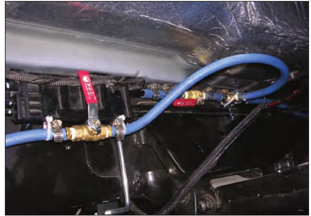
Stock valve is open, FASS valve is closed.
