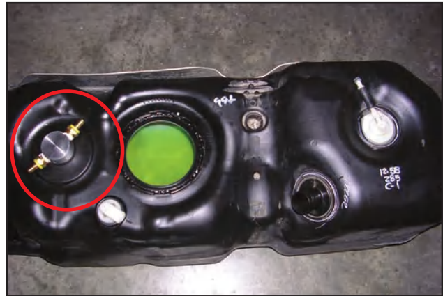
Here is a picture of the tank that has been removed from the truck. Look to the front and you can see the location of the new FASS drawstraw.
