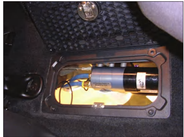
From above, a picture of the FASS unit that I installed on the outside of the driver's side frame rail.
