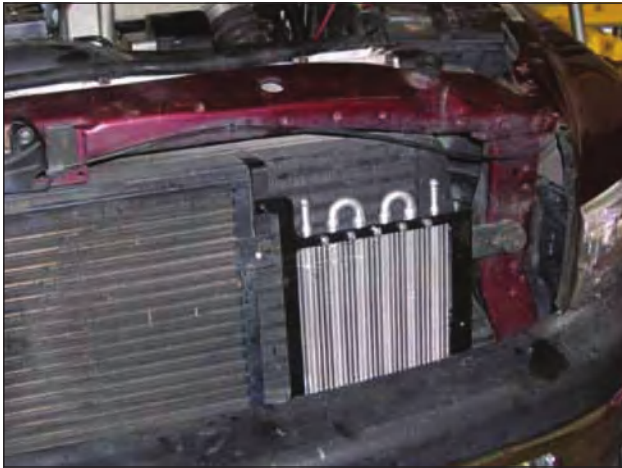
An automatic transmission fluid cooler in its new job as a power steering fluid cooler.
