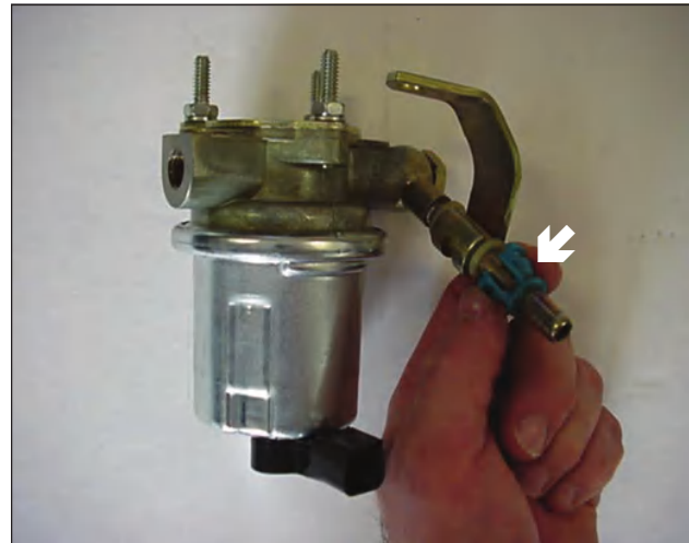
Pinch the blue disconnect and the fuel line will come loose.
