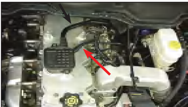
The 2003 crankcase vent system. The white arrow shows the inlet from the crankcase to the filter assembly. The red arrow points to the outlet hose that vents to atmosphere.
