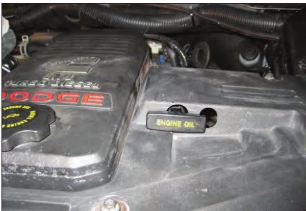
Modified "bat wing" with new dipstick location.
