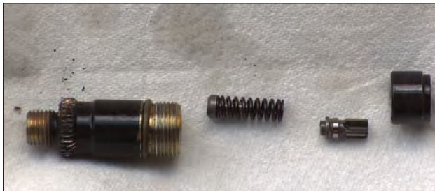
T8. Delivery valve parts removed from #1 injection pump barrel assembly in order to set timing.
