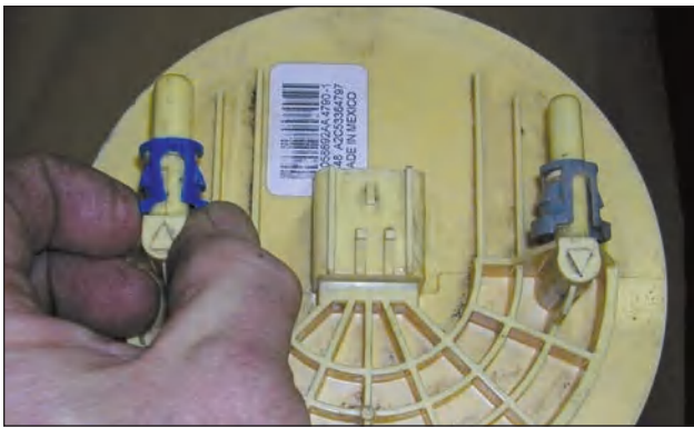
The pesky “pinch-in” clips that hold the fuel lines to the fuel pump assembly.
