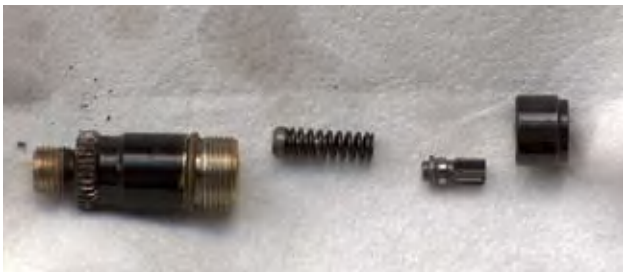
T8. Delivery valve parts removed from #1 injection pump barrel assembly in order to set timing.
