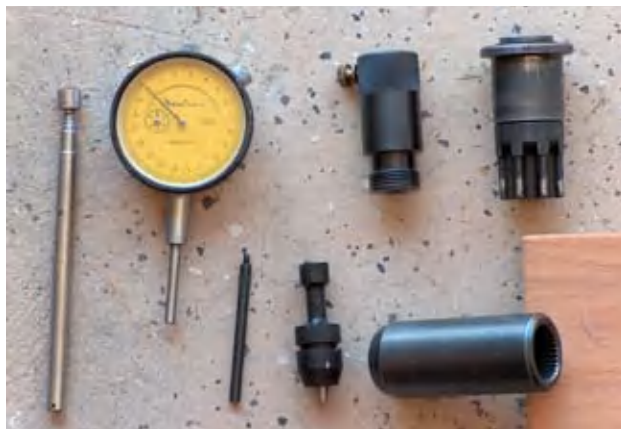
T5. Miller MLR-6860 P7100 pump timing tool kit. At the left is a magnet on a telescoping “stick.” To its right is the dial indicator with the stem extension below and to its right. To the right of that is a timing pin with a steel tip epoxy glued onto it. The special splined socket is at bottom right, with the splined end resting on a block of wood. At top center is the adapter that holds the dial indicator and screws into the top of the pump barrel. At top right is an engine barring tool that plugs into the aluminum block adapter plate and meshes with the flywheel teeth.
