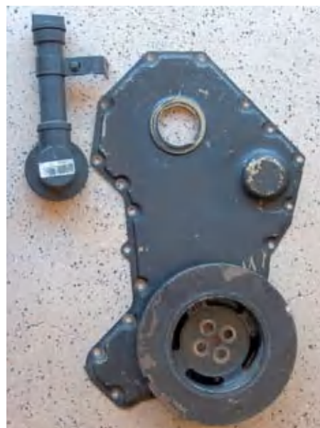
T10. A Cummins gear housing, front side, with the oil filler tube at top left.
