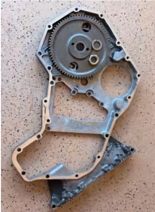
T11. A Cummins B gear housing with a P-pump drive gear, washer, and nut.
