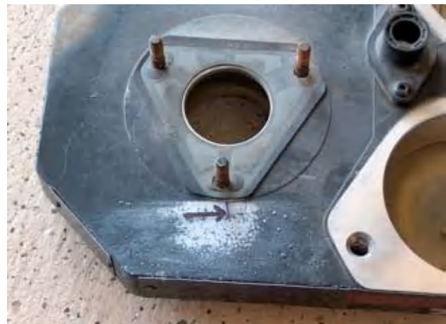
Close up view of the VE pump mounting area of the gear housing with the housing timing mark and the pump-to-housing gasket.
