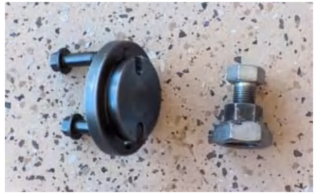
T6. The Snap-on SP504 gear puller with M8x1.25x40 bolts and the home-made pump shaft turning tool at right.
