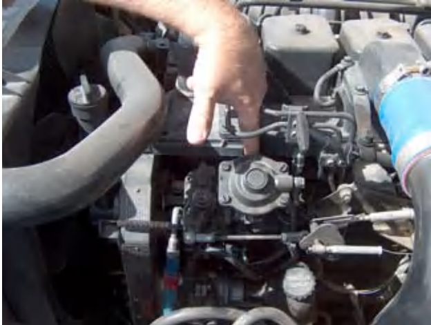
A Bosch VE pump on a Cummins B engine, with a finger showing the clearance between the AFC module and the cylinder head.
