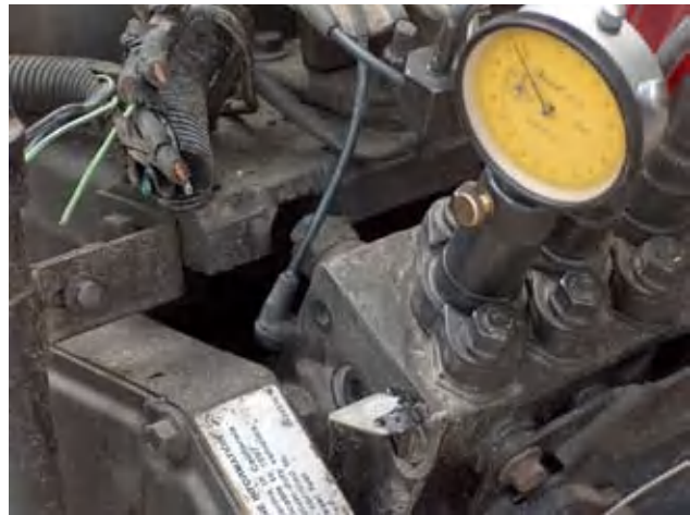
T9. Dial indicator installed in #1 barrel of a P7100 injection pump.
